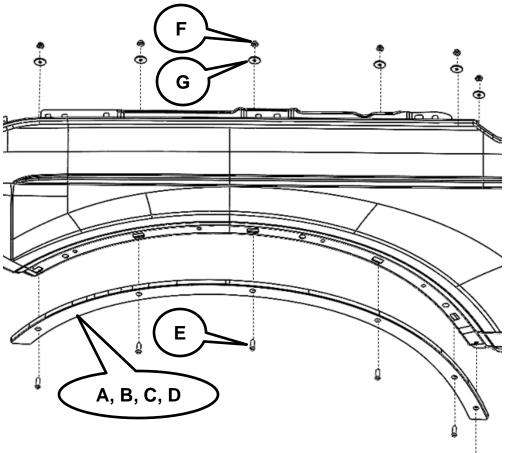
It will be necessary to remove the plastic screws from the felt fender well to access the back side of the fender to install washers (G) and nuts (F). Once fender delete (A, B, C, D) is installed, reinstall plastic screws to hold fender well in place.
